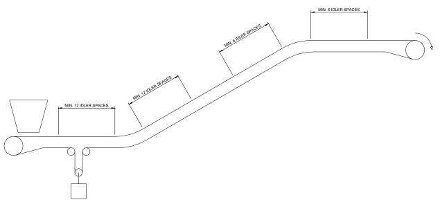
Position the weigher in the conveyor away from hoppers, chutes and transfer/transition points so that there is no movement of the material relative to the belt at all loading conditions.
