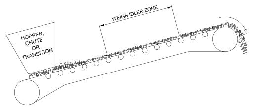
To facilitate routine weigh idler alignment and maintenance, ensure the weigh idler zone is at least one idler spacing clear of impact idlers and material (or Champion) skirts.
