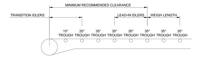
At any pulley with transition idlers, ensure the weigh length is a minimum recommended clearance of the greater of:
