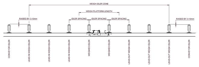
To ensure alignment, weighers should be aligned using 6 alignment wires on installation and as part of the routine calibration procedure.
