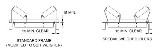
It is recommended that both the weigh rollers mounted on the belt weigher, the lead-in and lead-out rollers be balanced and machined. Our recommendation is that the roller be balanced to 0.014Nm and roller shell machined to 0.19mm total indicator run-out (T.I.R). Roller shafts should be fitted with an alignment locking screw both ends of the shaft to facilitate alignment.
