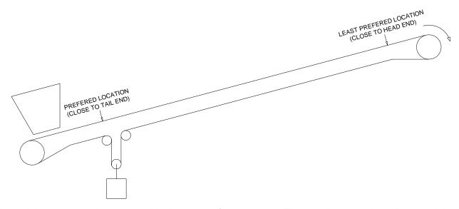
The weigher must not be mounted in the curve of a conveyor. The weigher must be at least 12 idler spaces from the end of a concave curve and 6 idler spaces from a convex curve.
